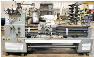
H.E.S. Type 550, 20" Geared Head Engine Lathe, S/N 12854, Finishing Stone Attachment, Tail Stock, Work Light
