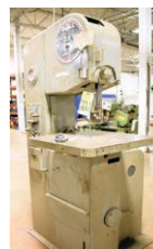
DoALL Model 1612-0, 16" Vertical Contour Metal Cutting Band Saw, S/N 209-64512, with DoAll DBW-12B Blade Butt Welder, S/N 211-64483
