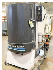
HOTSY Model 7530, Enclosed 2-Tier Rotary Carousel Parts Washer, S/N 5001379 (2002), 3-HP Motor, 1-PH
