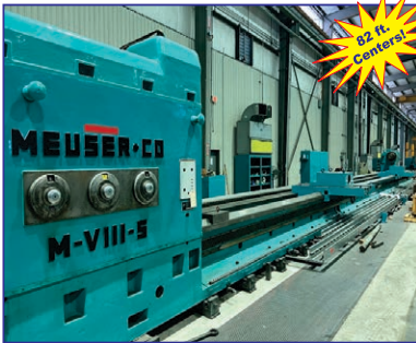
86" x 984" Meuser Model M-VIII-S CNC Lathe (Retrofit)
